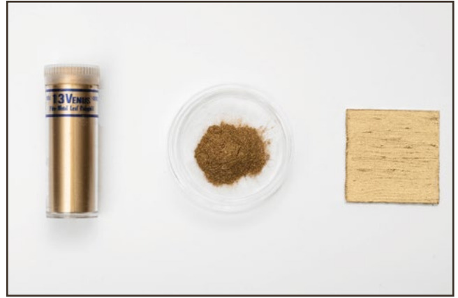
Pictured here are sample materials used by The Andy Warhol Museum staff to create mock-ups of Oxidation for testing. The container on the left of the image contains Venus Bronze Powder Pale Gold No. 13, one of several metallic powders Warhol would have used in creating his Oxidation paintings. (Photo: Bryan Conley)
