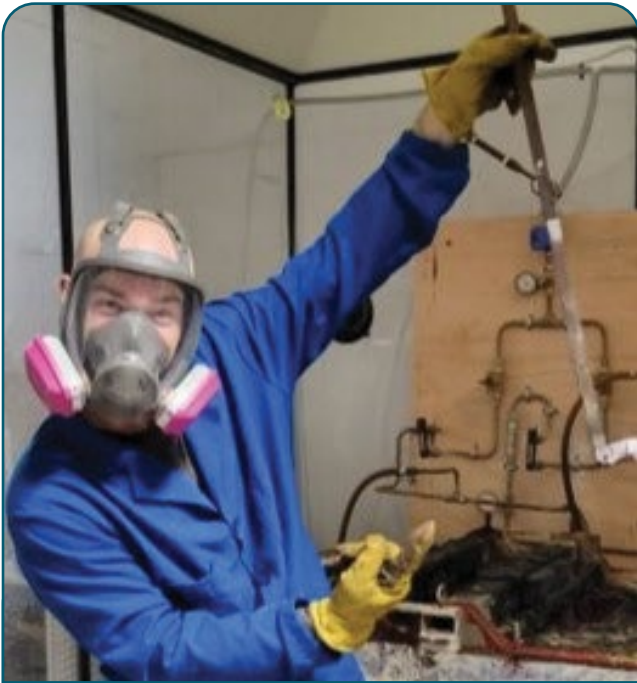
A technician removing magnesium from Magrathea's pilot electrolyzer.
