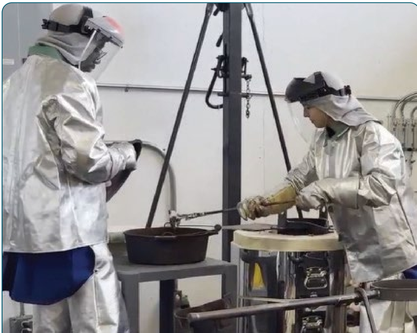
Technician team pouring ingots in Magrathea's pilot foundry. Photos provided by Magrathea.
