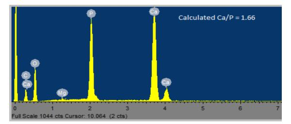
Figure 1: EDS spectra of the HAp product with Ca/P ratio 1.66 prepared using eggshells calcinated at 800°C after heat treatment by 1M H<sub>3</sub>PO<sub>4</sub>
