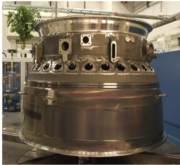
Figure 4. A René 220 casting (upper complex geometry CRF part) joined by EB-welding to a wrought alloy 718 skirt.
