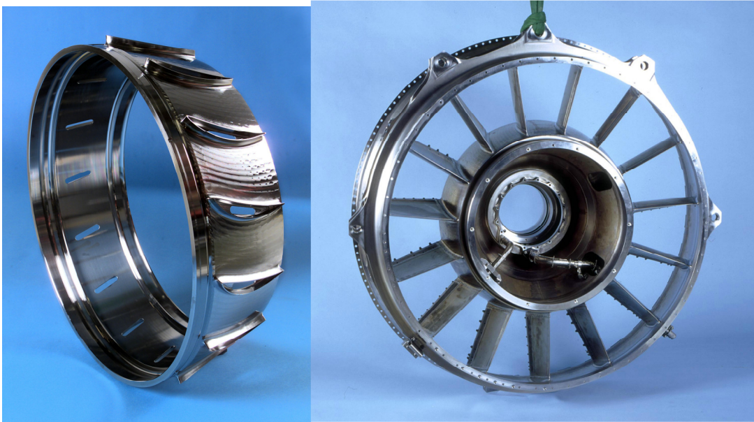
Figure 7. A “traditional” assembly part - a turbine exhaust case in Greek Ascoloy material. The milled wrought (ring rolled) inner and outer rings are joined by sheet metal struts.
