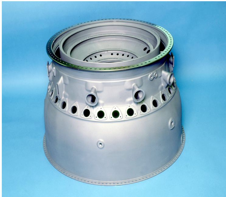
Figure 3. A compressor rear frame (CRF) as an Alloy 718 one-piece casting. Cast on flanges have been replaced for strength with wrought rings and joined by EB-weld to the cast main body. The structure here is shown after final machining.
