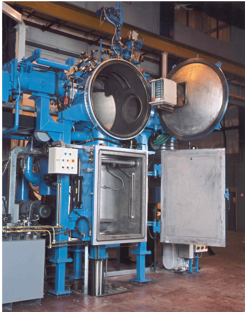
Figure 2. Two chamber batch type vacuum investment casting equipment for equiaxed investment castings. The melting of the feed stock material (usually a piece of a bar) is done in a crucible by the induction coil lining the crucible (visible as attached to the swing door of the top chamber). The lower chamber is in the open position to receive the externally preheated casting molds. Courtesy Consarc.
