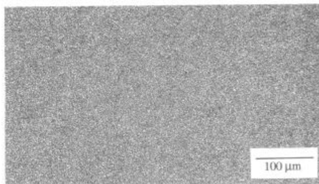
Figure 2. As-deposited microstructure of RD-8A alloy.
