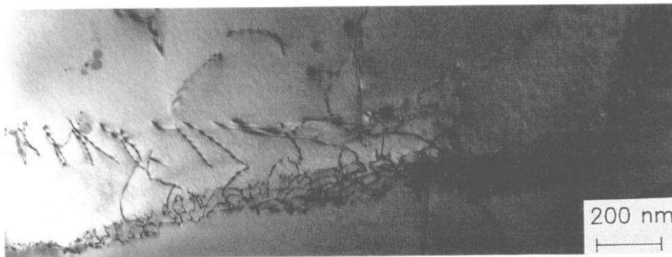
Fig. 7 TEM micrographs (bright field) of dislocation networks at the \gamma/\gamma' interface in an creep tested specimen (110 MPa, 7.6 %, 950 °C)
