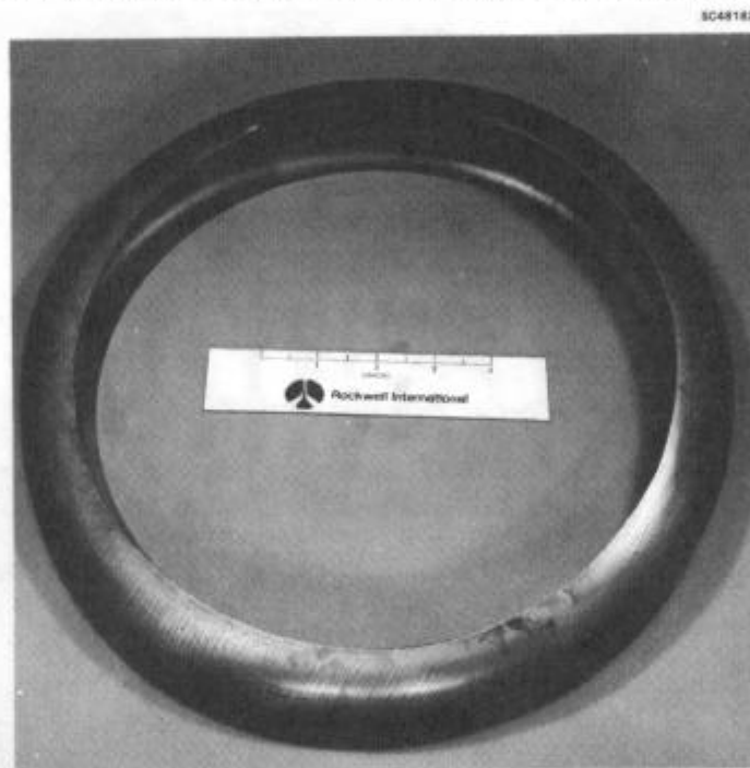
Fig. 11 Alloy 718 tested at 982^\circ C and 5 \times 10^{-4}/s with increasing superplastic strain.
