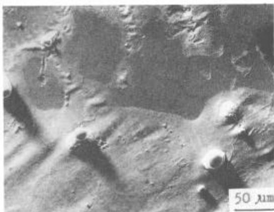
Figure 4 -- Liquid film and spherule of alloy DZ22.
