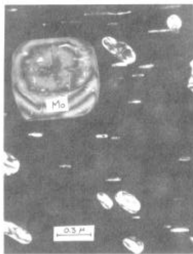
Photo. 4 Mo Platelets in \gamma/\gamma' - \alpha Quenched and Aged at 900°C x 10h
