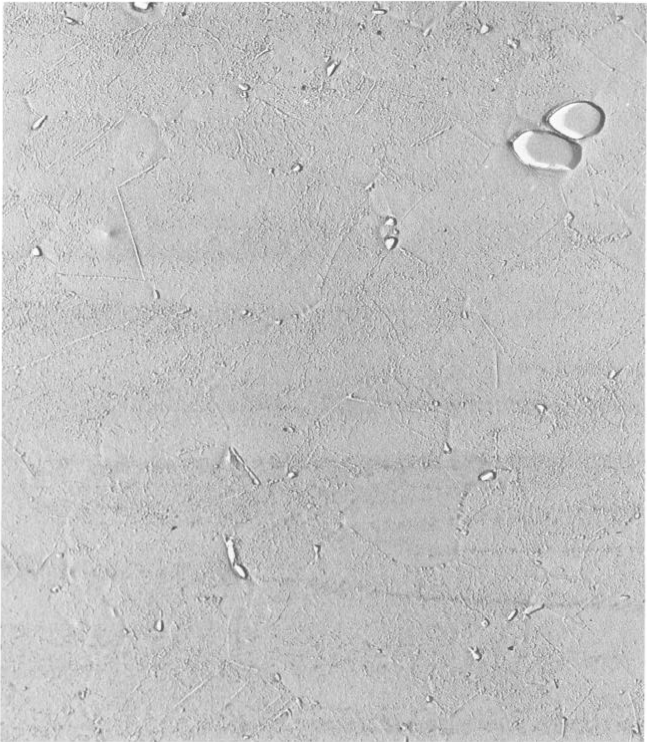
Figure 5. Electron Microstructure of Inco 718 as-forged at a slow rate from a 1825° F. initial temperature. 25,000X
