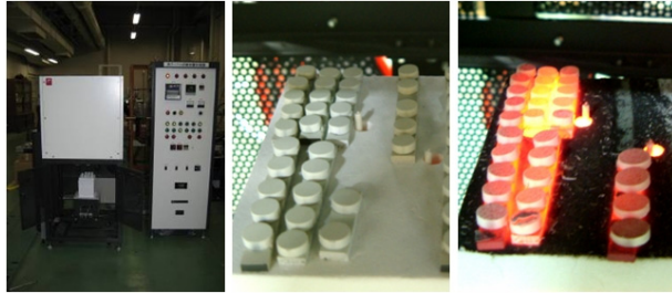
Figure 1. Pictures showing the use of the thermal cycling furnace (left), the placement of specimens on the sample stage (centre) and the heating/cooling conditions (right).
