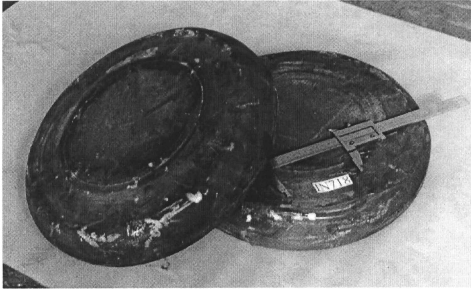
Figure 6. Photographs of the alloy 718 forgings that were produced by upset forging at temperatures of 900 to 975°C.
