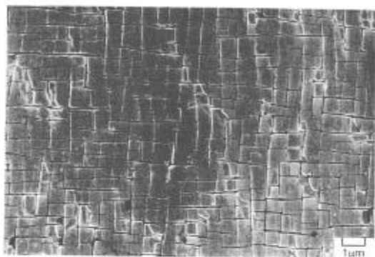
Fig. 1. Scanning electron micrograph of a single crystal nickel-based superalloy, CMSX-4.
