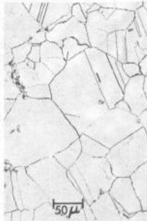
ASTM Grain Size 5 Fig. 15. Cross rolled ESR hollow section.
