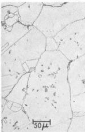
ASTM Grain Size 1 1/2 Fig. 14. Upset forged photomicrograph.
