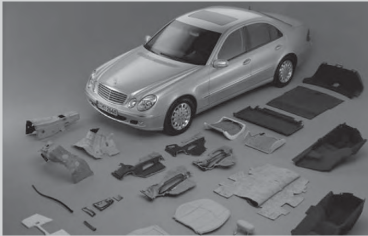
Figure 1. Automobile components made of natural-fiber-reinforced composites. 25
