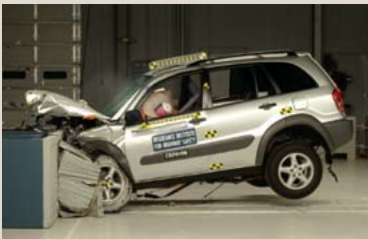
Crash test – courtesy Insurance Institute for Highway Safety
