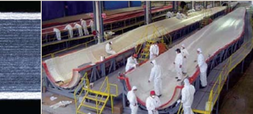
Wind turbine blade manufacture – courtesy TPI composites
