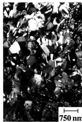
Figure 2. Microstructure of the alloy 718 after forging at a strain rate of 5.5 \times 10^{-3} \text{ s}^{-1} and 850^\circ\text{C} to generate an MC structure.
