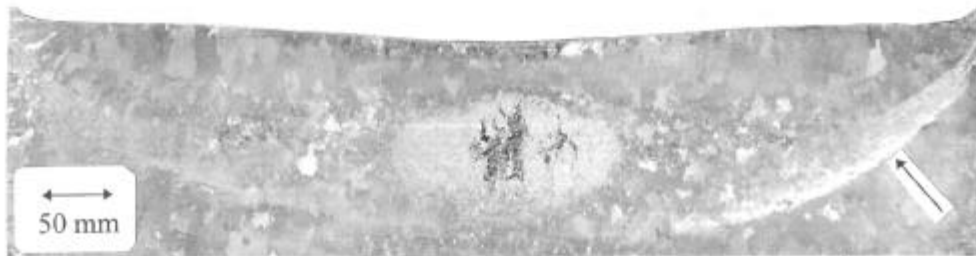
Figure 2. Pool Profile for 686 mm Diameter Ingot Melted at the Optimum Rate
