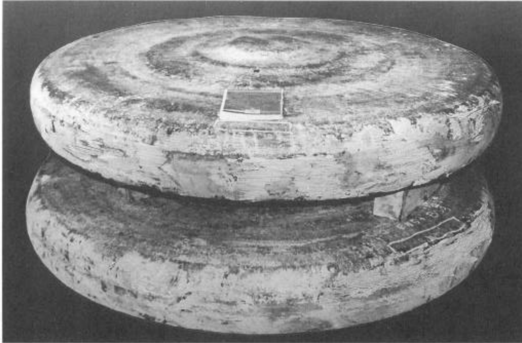
Figure 10. Full Size (2000 mm Diameter) Alloy 718 Disks
