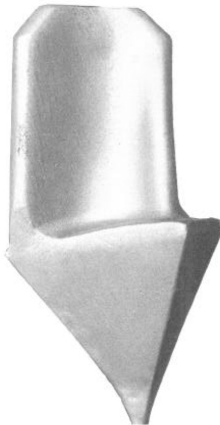
Figure 14. Single crystal NiAl castings of a large HPT blade shape.
