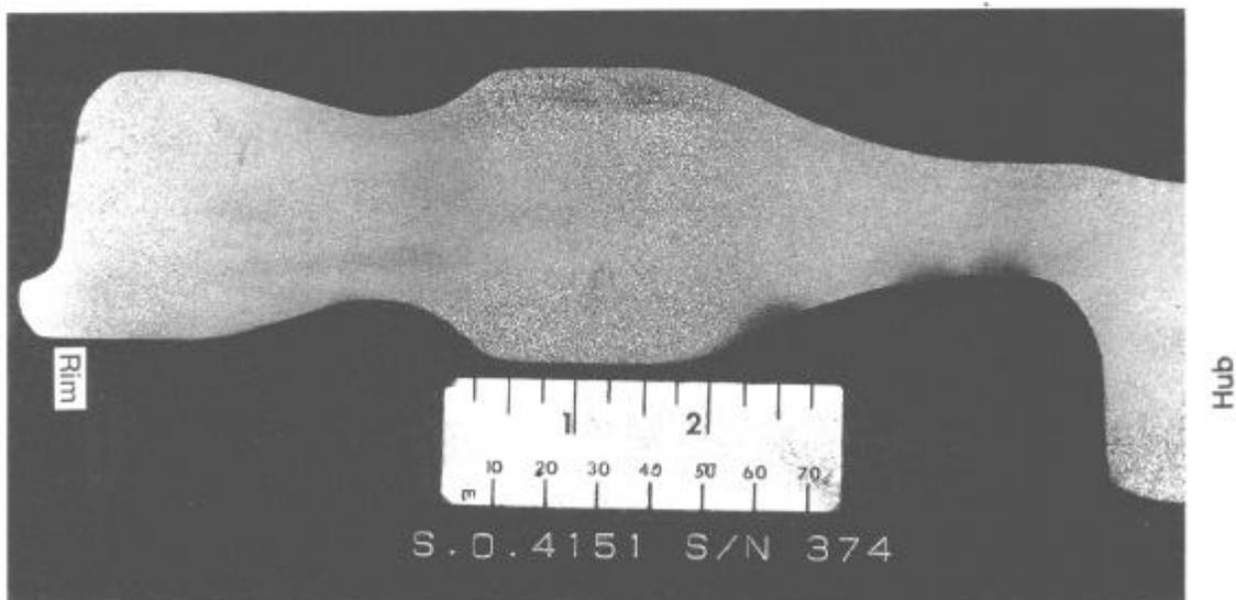
Figure 1.—Low cobalt waspaloy forging.
