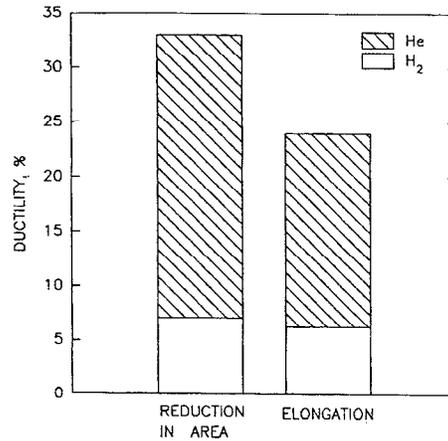
Figure 13.—Effect of high pressure H<sub>2</sub> on the ductility of low cobalt waspaloy.
