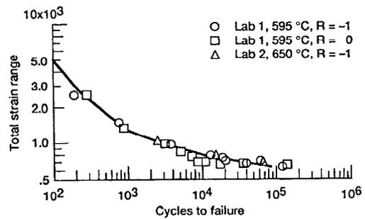
Figure 9.—Low cycle fatigue behavior of low cobalt waspaloy at 595 and 650 °C.
