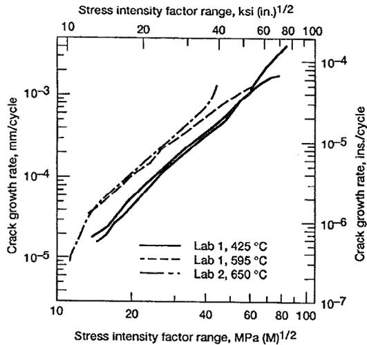
Figure 11.—Cyclic crack growth behavior of low cobalt waspaloy.
