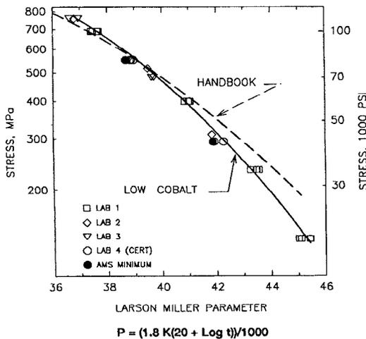
Figure 6.—Stress rupture of low cobalt waspaloy.
