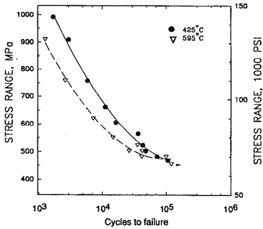
Figure 10.—Load controlled low cycle fatigue of low cobalt waspaloy.
