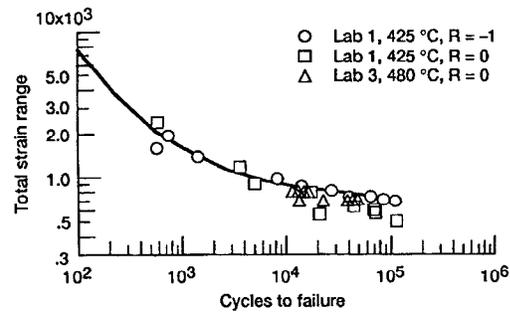
Figure 8.—Low cycle fatigue behavior of low cobalt waspaloy at 425 and 480 °C.
