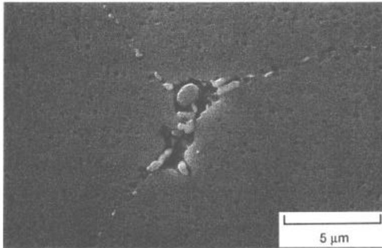
Figure 3.—Scanning electron micrograph of low cobalt waspaloy.
