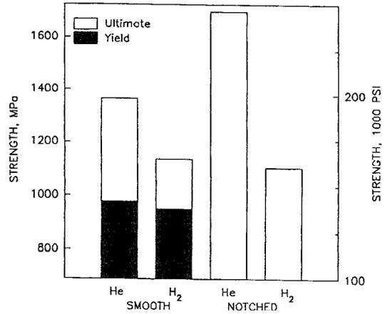
Figure 12.—Effect of high pressure H<sub>2</sub> on the tensile strength of low cobalt waspaloy.
