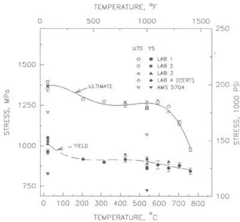
Figure 4.—Effect of temperature on the strength of low cobalt waspaloy.
